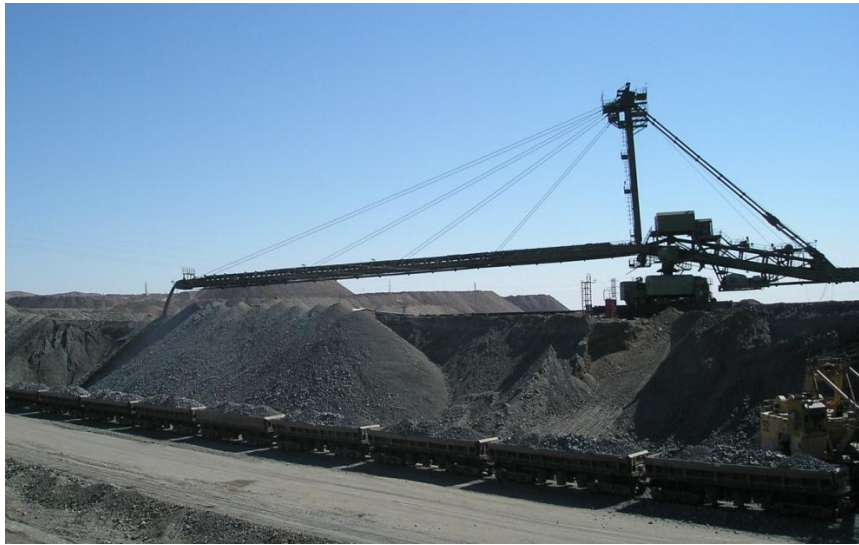
Illustration 2. Ore dumping with the OSS 4000/125 cantilever dumper and loading of EKG-10 commercial ore into railway dumpcars
