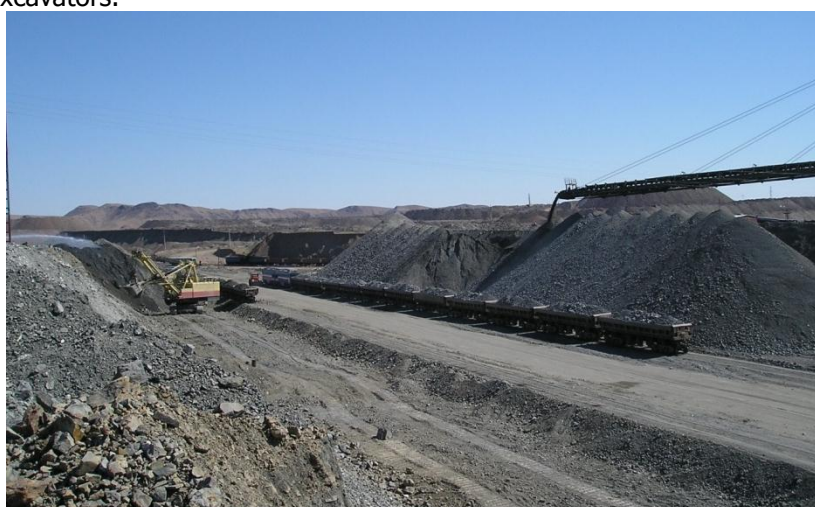
Illustration 1. Loading of EKG-10 commercial ore into railway dumpcars
